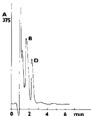
Fig. 6. Chromatogram of an irradiated solution of bilirubin in phosphate buffer of pH 8.25. Concentration of bilirubin,  $39 \mu\text{mol/l}$ ; concentration of riboflavin,  $5 \mu\text{mol/l}$ ; flow-rate after 20 min irradiation,  $1.0 \text{ ml/min}$ ; mobile phase, Tris buffer of pH 6.0 + 80% methanol. The chromatogram shows the formation of biliverdin dimer.
