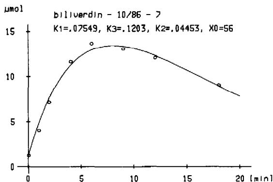
Fig. 5. Experimental and calculated curves for biliverdin formation in a buffer of pH 6.8. Concentration of bilirubin with albumin,  $56 \mu\text{mol/l}$ ; concentration of riboflavin phosphate,  $5 \mu\text{mol/l}$ ; irradiated in a 0.5-cm cuvette with sunlight. Rate constants:  $k=0.12002$ ;  $k_1=0.07549$ ;  $k_3=0.1203$ ;  $k=k_1+k_2$ .
